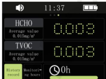
※The monitoring time must be longer than 1 hour, and the measured data will be of reference significance.
