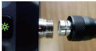
Connect soft cable port with the host port (indicating the alignment of the mark) and turn it clockwise until it locks.
